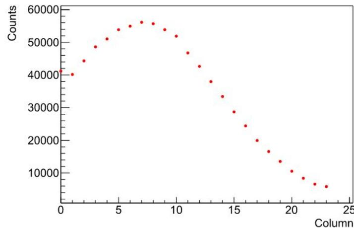
Fig. 25. In the adder readout mode, the sum of all counter states per column is read out. The result is a projection. The graph shows the profile of a carbon beam with  $2 \times 10^6$  ions/s at an energy of 423.44 MeV/u, measured by HitPixS.
