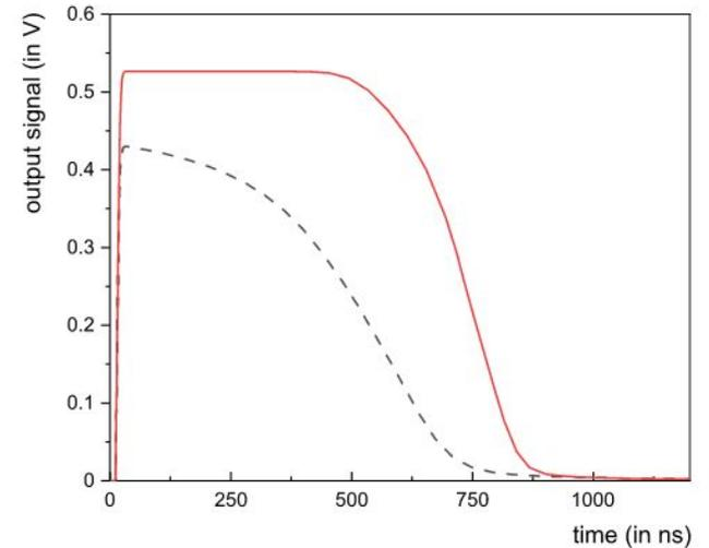
Fig. 14. Simulation of the HitPixS amplifier to an input signal of  $27800 e^-$  (dashed line) and  $3 \times 27800 e^-$  (solid line).
