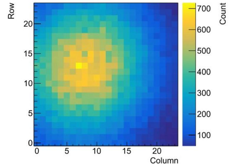
Fig. 26. Integrated counts of the pixels displaying the spot of the carbon beam  $2 \times 10^6$  carbon ions/s at an energy of 430.10 MeV/u. Measured on HitPixISO.
