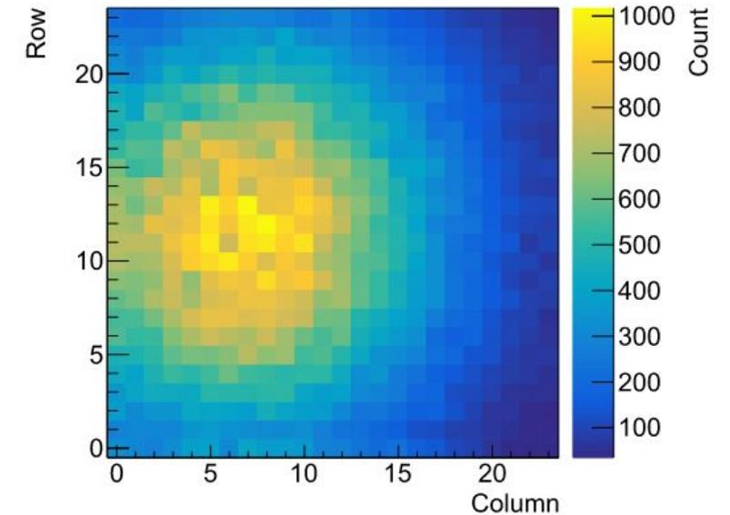
Fig. 24. Integrated counts of the pixels displaying the spot of the carbon beam  $2 \times 10^6$  carbon ions/s at an energy of 423.44 MeV/u. Measured on HitPixS.
