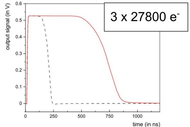
Fig. 15. Simulated signal length for a feedback current of 0.5 nA (solid line) and 2.5 nA (dashed line).
