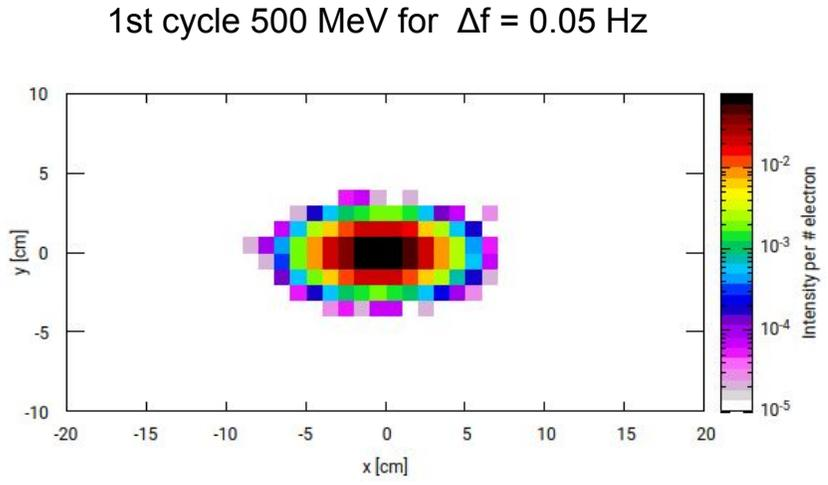
Current beam with energy of 500 MeV measured with beam camera
