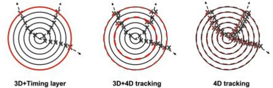
Figure 2: Possible implementations of a tracker system with timing capability.
