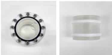
The plastic scintillator was coiled with thin Teflon to fix it inside the PTFE container. The liquid scintillator was shelled up after fixing the plastic scintillator.
