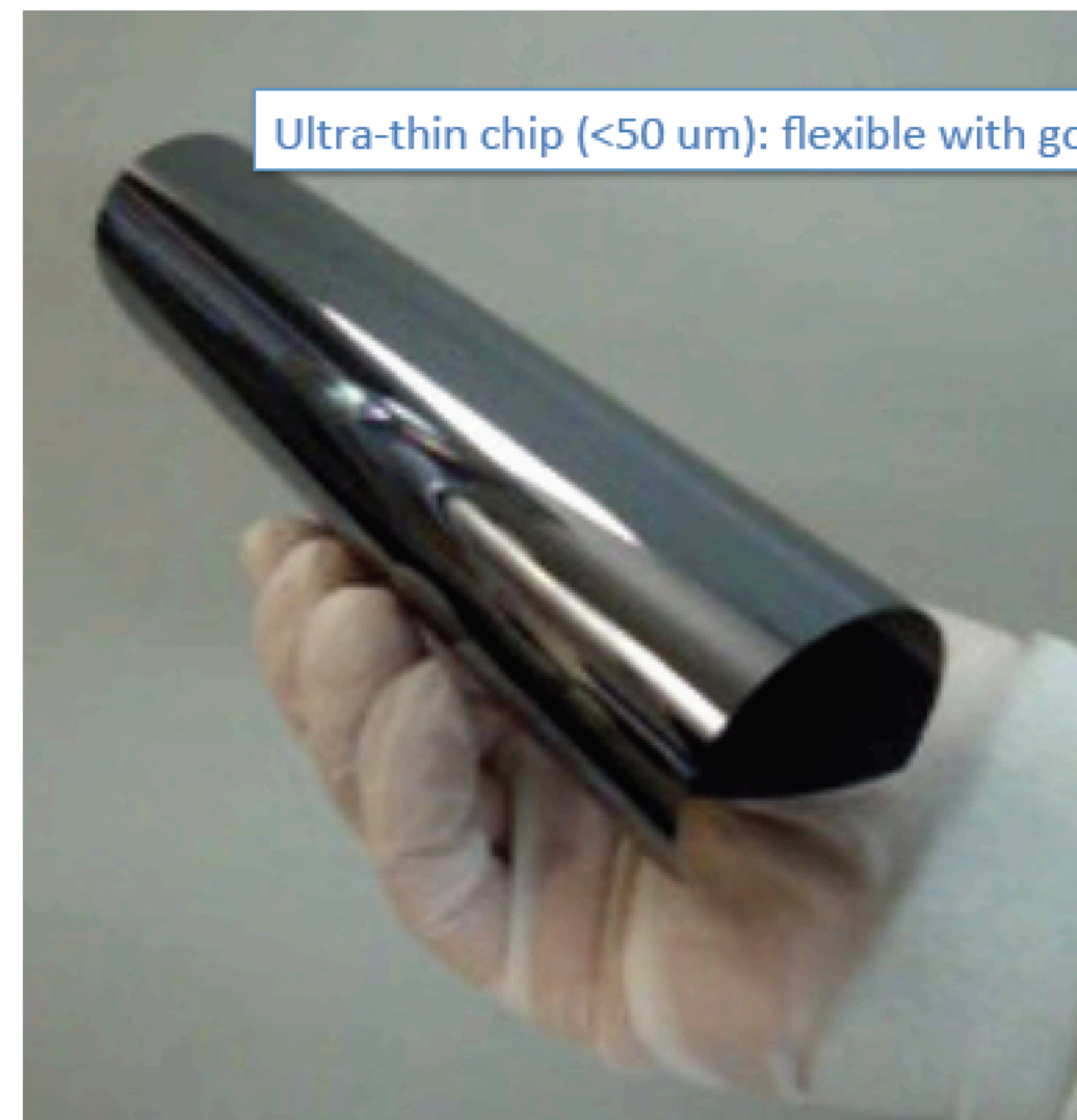
Silicon Genesis: 20 micron thick Si wafer
