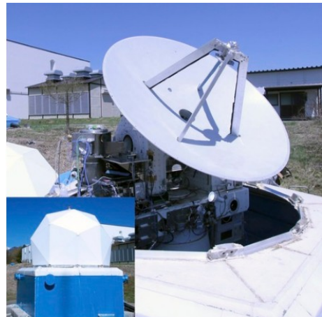
The 1.85m mm/sub-mm telescope (Osaka Prefecture University). 12 CO, 13 CO, and C 18 O (J = 2-1); 230 GHz; 3 arcmin; -100 to 80 kms -1 rms ~0.3K at a 0.3 kms -1 .
